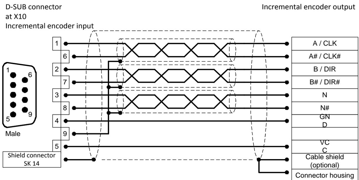
Figure 14: Pin assignment: Incremental Encoder Input [X10]
