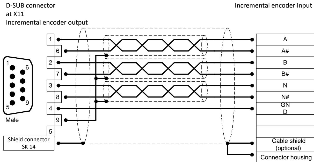
Figure 15: Pin assignment: Incremental Encoder Output [X11]
