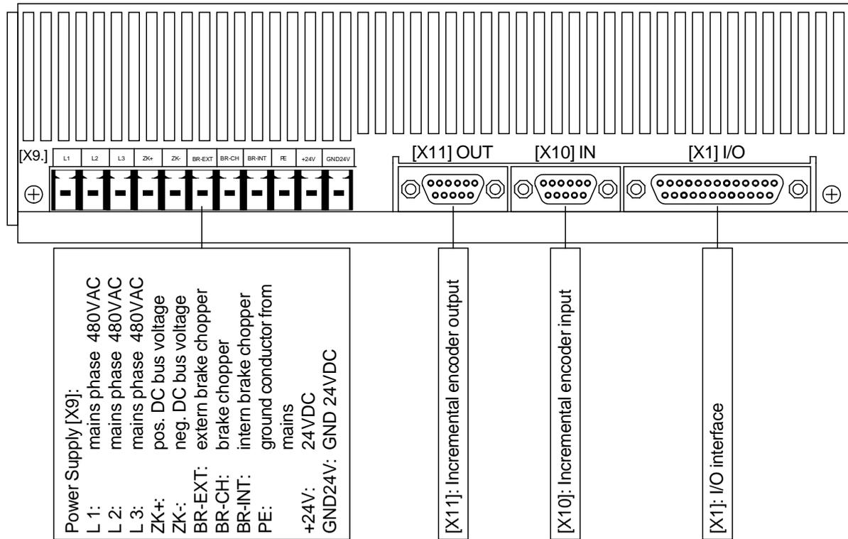
Figure 2: Servo drive ARS 2302 SE: Top view
