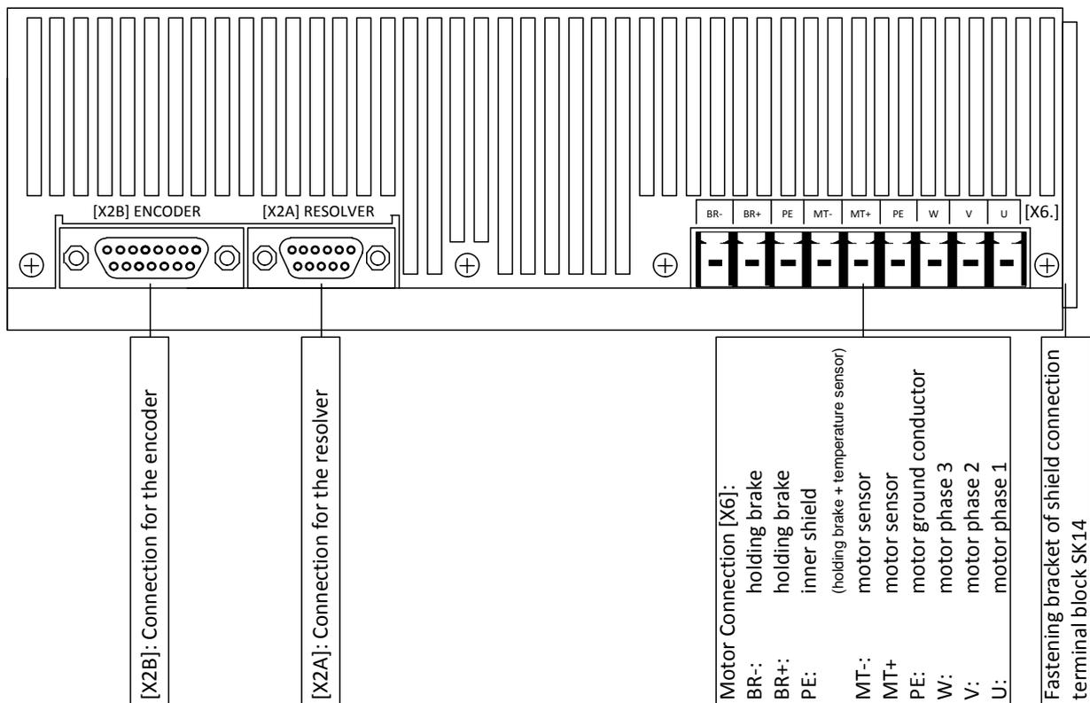
Figure 3: Servo drive ARS 2302 SE: Bottom view
