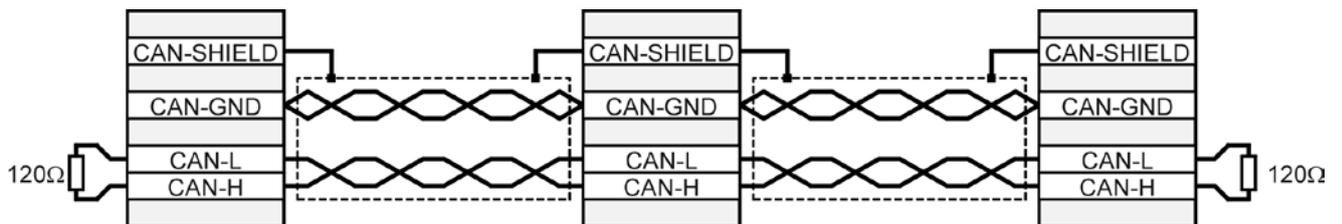
Figure 10: CAN bus cabling example
