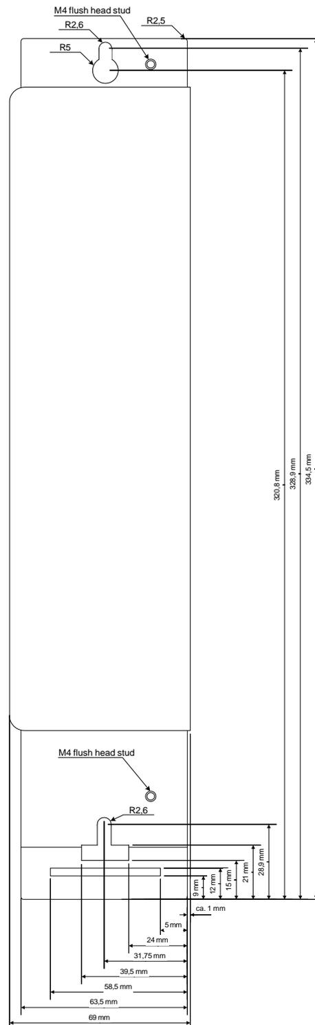
**Figure 4: Servo drive ARS 2300 SE: Mounting plate**
