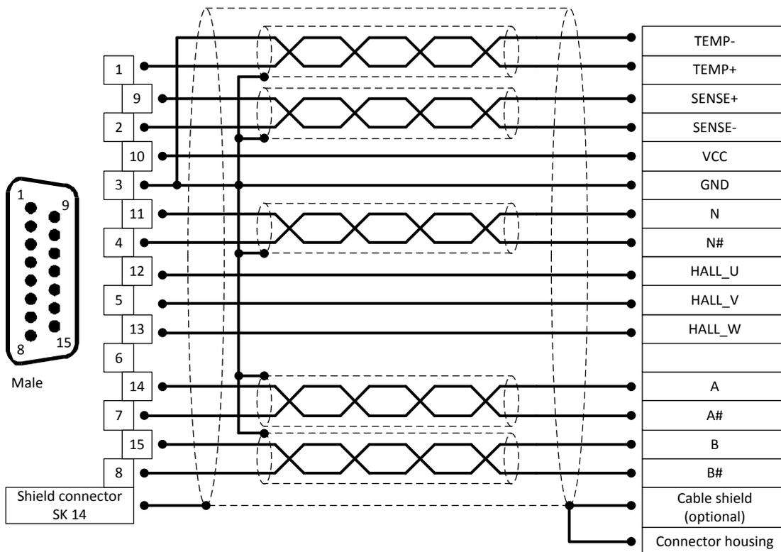
**Figure 9: Pin assignment: Digital incremental encoder [X2B]**
