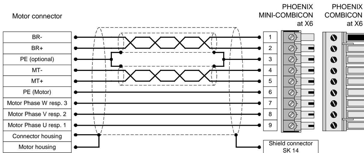
**Figure 13: Motor connection [X6]**
