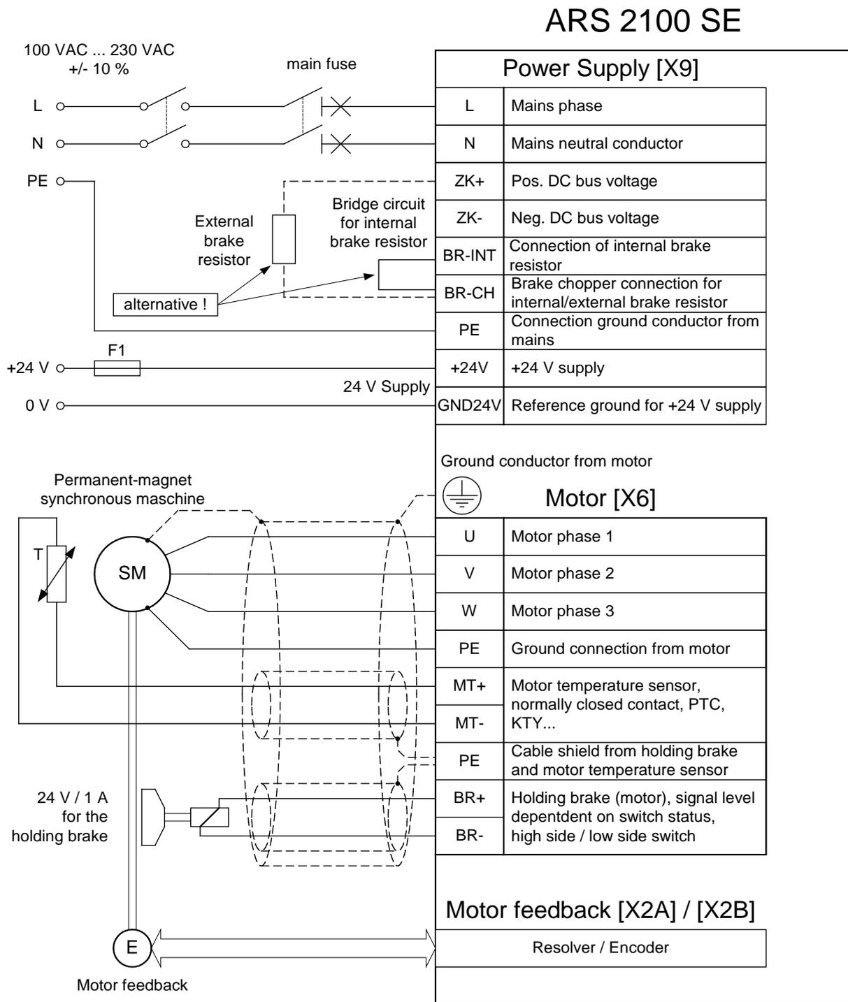
Figure 11: Connection to power supply [X9] and motor [X6]
