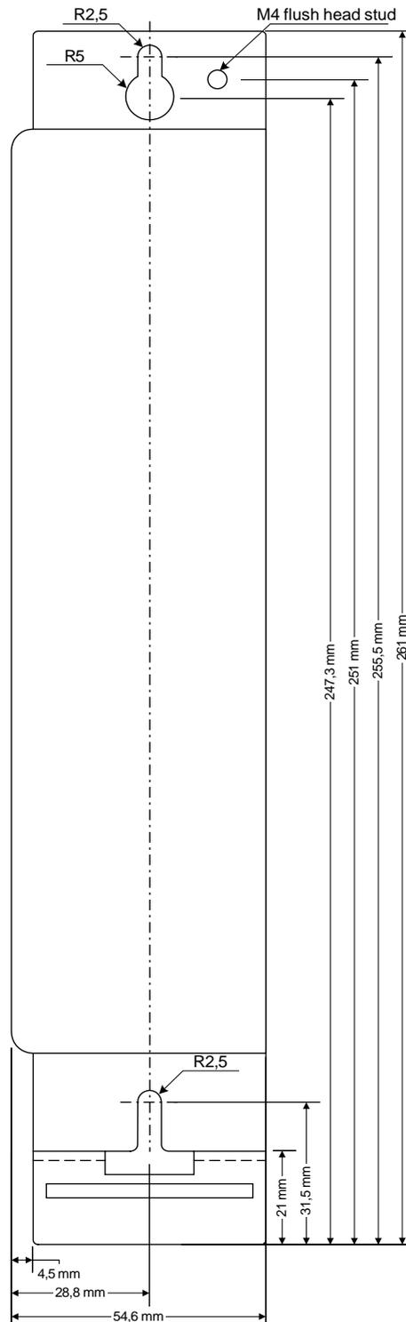
**Figure 4: Servo drive ARS 2100 SE: Mounting plate**
