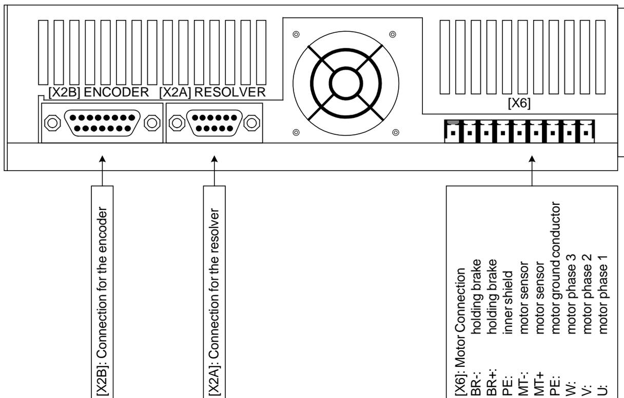
Figure 3: Servo drive ARS 2102 SE: Bottom view
