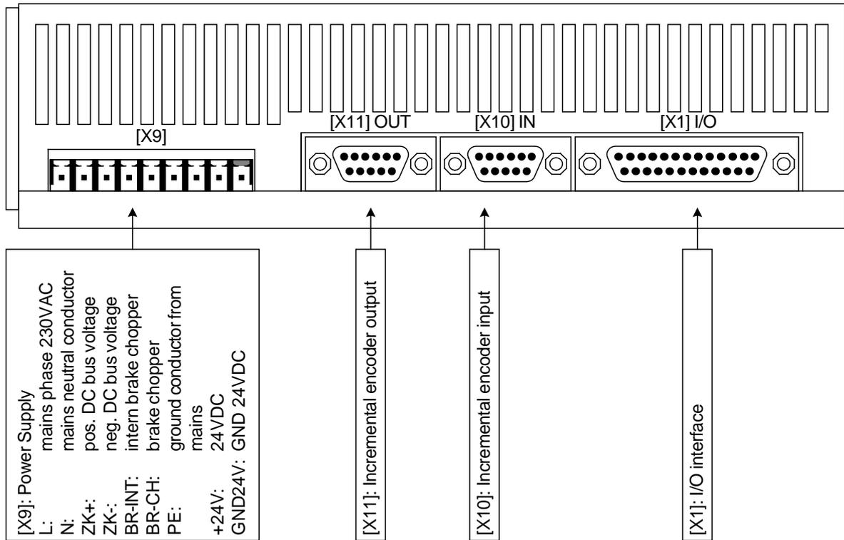
Figure 2: Servo drive ARS 2102 SE: Top view
