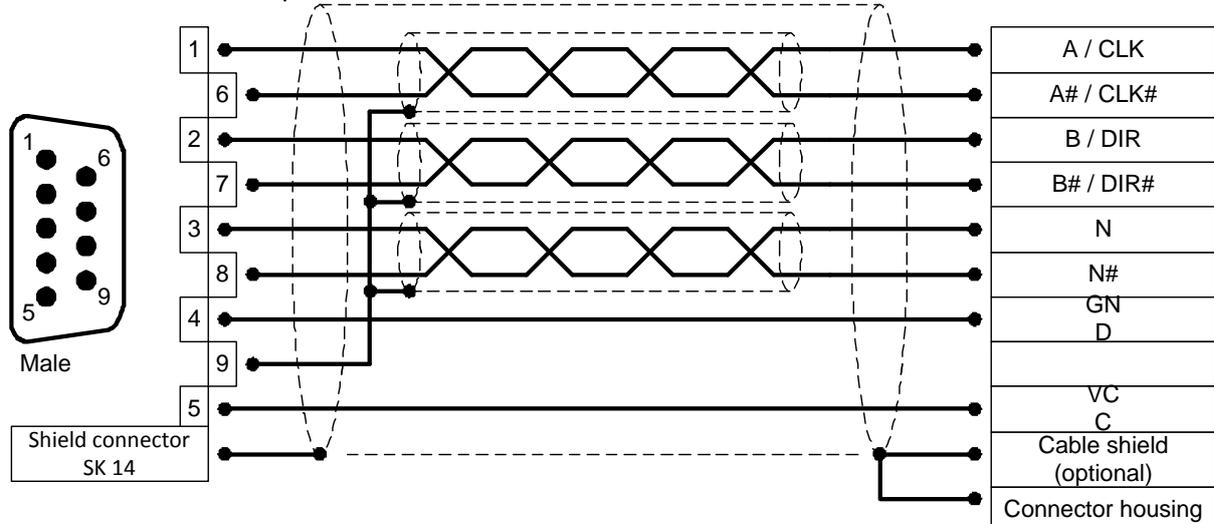
Figure 14: Pin assignment: Incremental Encoder Input [X10]
