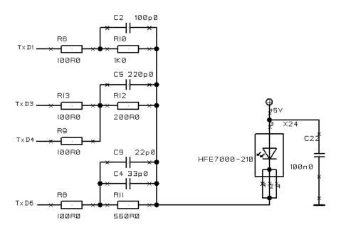
Figure 11.18: Connection of transmitter diode
