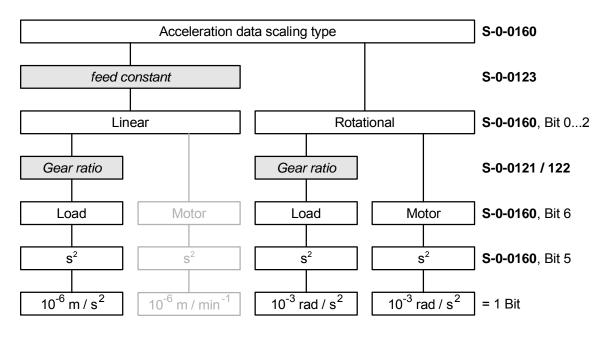
Figure 9.14: Acceleration data scaling
