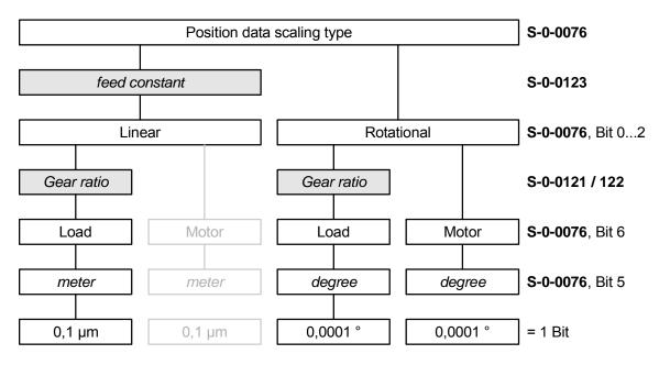
Figure 9.12: Position data scaling
