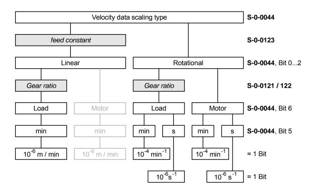
Figure 9.13: Velocity data scaling
