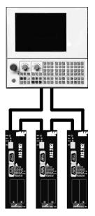
An optical fiber ring is used as transmission medium. The transmission rate is 2, 4, 8 or 16 Mbit/s.
