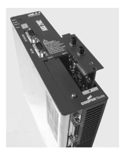
Figure 3.2: Plug-in position for ARS 2102, 2105, 2302, 2305 and 2310
