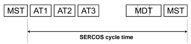
Figure 5.5: Cyclic data exchange
