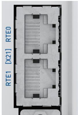
Figure 1: Connector view fieldbus interface BL 4000-C
