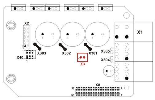
Figure 28: Position and connection holding brake
