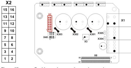
Figure 27: Position and connection angle encoder
