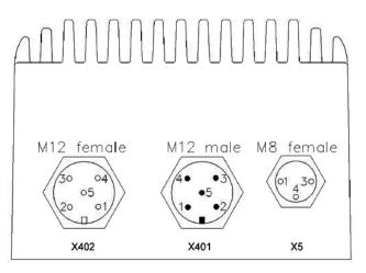
Figure 32: Position and connection RS232 interface
