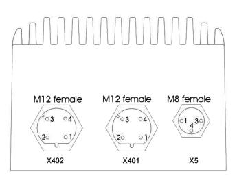
Figure 35: Position and connection EtherCAT interface
