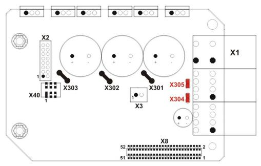
Figure 29: Position and connection brake resistor
