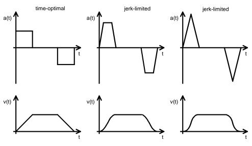
Figure 4: Motion profiles of the DIS-2 48/10 FB FS STO
