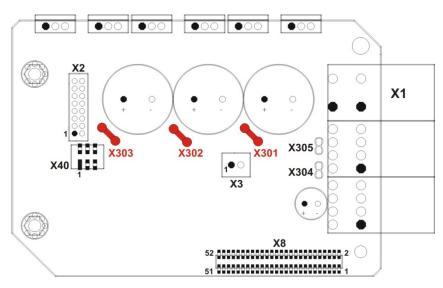
Figure 26: Position and connection motor cable
