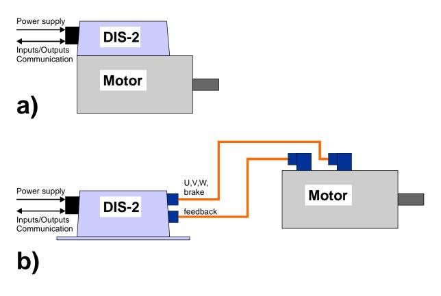
Figure 17:a) Mounted directly on the motor – standard,b) Separated from the motor – Please contact your local distributor to checkwhether this option is available.
