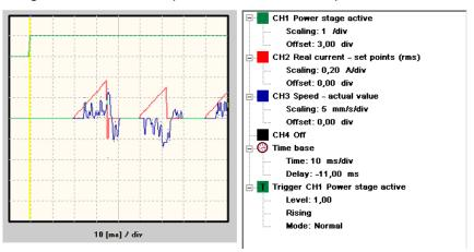
Basically the reduction causes a change in ramp steepness. The drive is operated with less acceleration but in return it needs a longer time for one step. The excitation at vibratory mechanic is smaller and therefore the measuring more approvable. Which value is more
