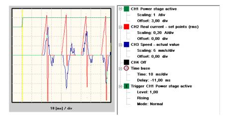
Though the curve of the current value of speed is interesting. The drive will accelerate due to the current rise and afterwards it will slowed down to speed 0 by an inverted current pulse. However at elastic assemblies these short pulses can lead to an oscillation of the mechanic as well as of the driving shaft. The measuring result will then be corrupted. The process does not provide a valid commutating position and will end with error 35-5.
